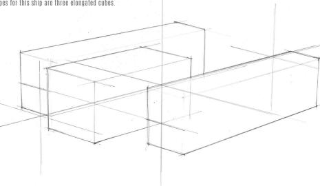
Begin to "carve out" the more refined shapes of the ship. The engines and cockpit module are going to be more aerodynamic, so cut some swept-back angles for the fronts of those. The exhaust cowling, just over halfway down the rear of each engine, is angled backwards. It's possible to approximate that these details will be symmetrical by measuring them against the perspective guides. Loosely rough in a sphere near the nose for the base of the weapon turret.
